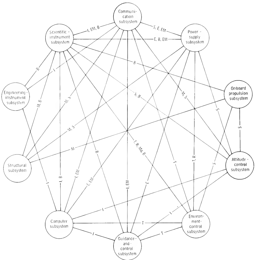
FIGURE 9-3.—Spacecraft-interface diagram. Only the major interfaces are shown: T =thermal, S =spatial, E =electrical, R =radiative, Ma =magnetic, I =information, B =biological, EM =electromagnetic, M =mechanical.
